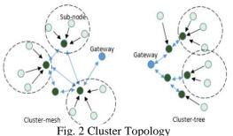
Clustering in network will make network become hierarchical and also improve the bandwidth utilization because only some dedicated nodes maintain connection on communication channels. In stationary WSN, clustertree topology has the best energy efficiency while clustermesh topology provides the maximum robustness which allows multi-path routing and multiple sinks.
